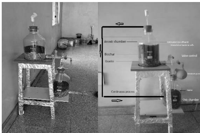
Fig 1: Fabricated Aerobic and Anaerobic Degradation Chambers with Biochar levels higher in the anaerobic chamber and designed for continuous batch fermentation
