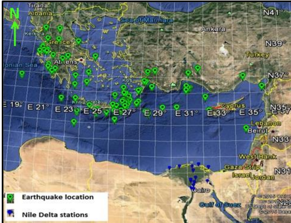
Figure 3 a map show Epicentral of earthquakes used in calculations after applying selection criteria
