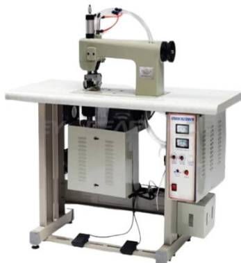
Figure(5): Ultrasonic sewing machine
