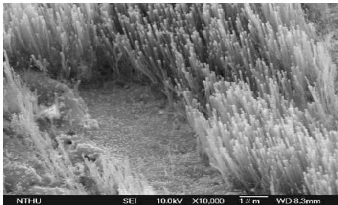
Figure 4 shows the SEM of (a) well-aligned and thriving CNT growth on a Cu-10 wt% Fe-10 wt% Co-10 wt% substrate. Substratum made of bulk nickel alloy, and (b) an illustration of the right side of (a) displaying upright tubes embedded with catalyst particles at tips. Reprinted from [53], S. Y. Chen et al., J. Phys. D.: Appl. Phys. 37, 273, with permission (2003). Institute of Physics, 2003.
