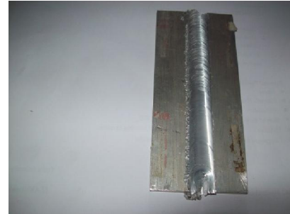
Figure 9.friction stir welded aluminum alloy H20 triangular tool
