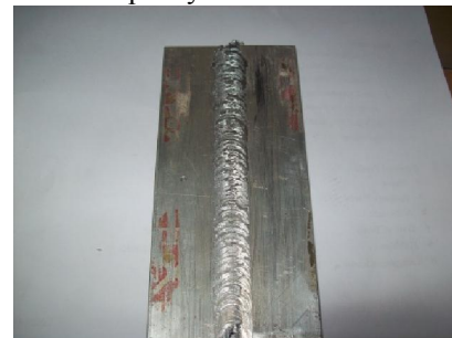
Figure 11. friction stir welded aluminum alloy H20 straight cylindrical tool.
