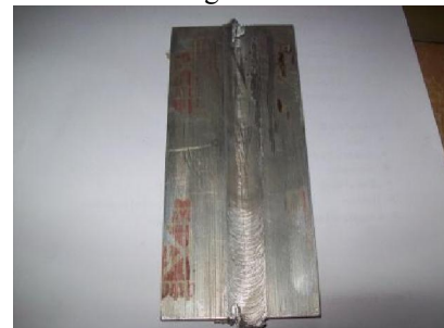
Figure 10. friction stir welded aluminum alloy H20 taper cylindrical tool.
