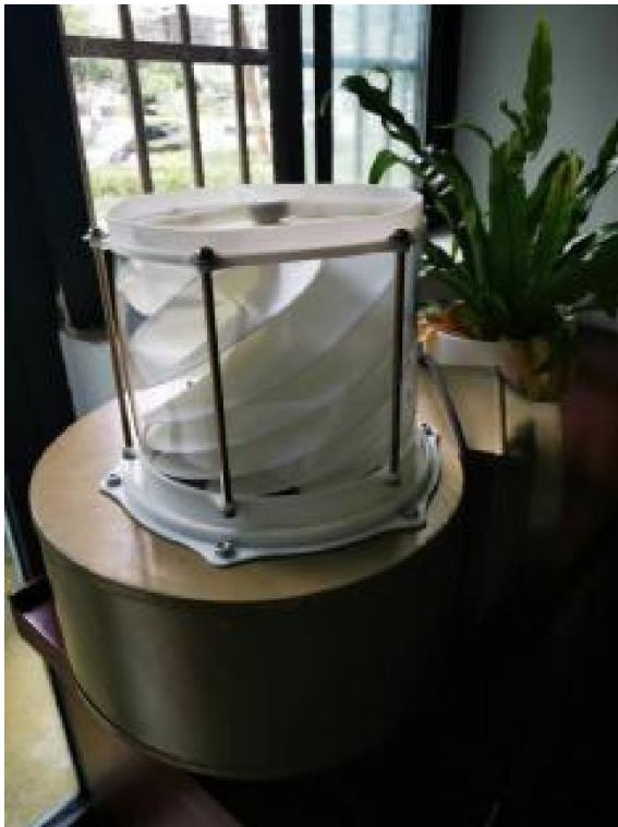
Figure 8. Scroll blade structure
