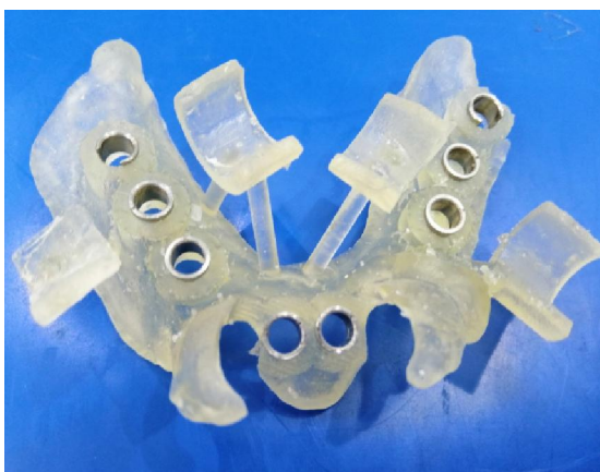
Fig. (5): The surgical guides were printed using a 3D printer.
