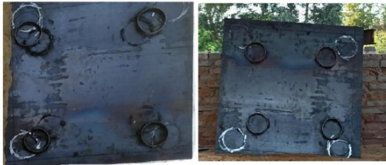
Fig (16) steel plate (with different diameters from center to center) – group of four piles
