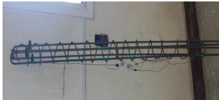
Fig (4) Internal strain gauges
