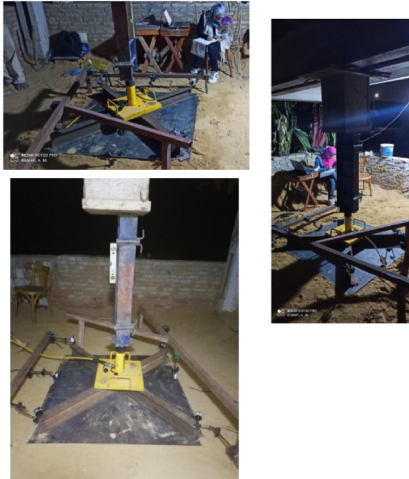
Fig (19) Reference beam and dial gauges setup for – group of four piles
