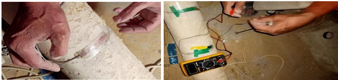
Fig (5) strain gauges on concrete
