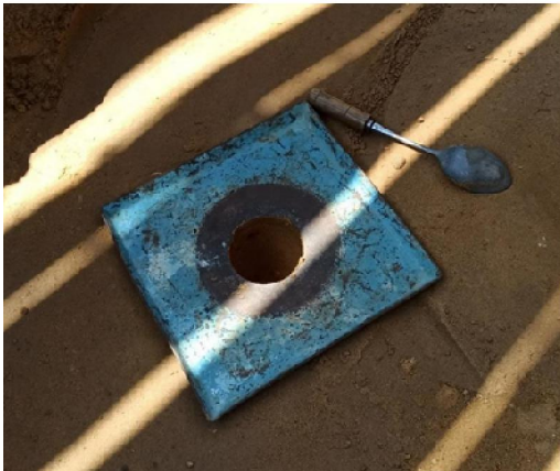
Fig (11) Sand cone test
