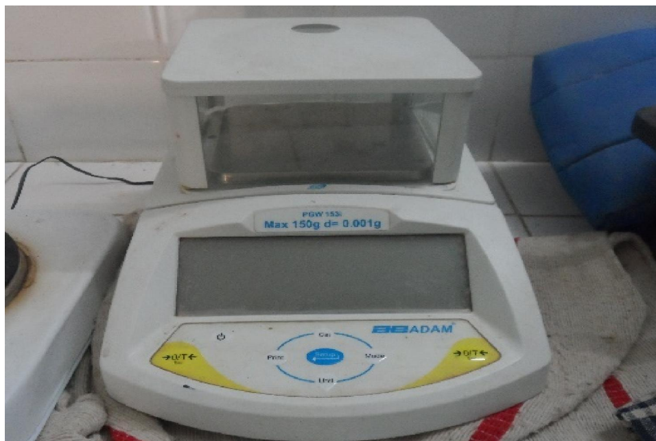
Photo indicate that the sensitive electronic scale used in weighting the dried Erucasativax sample
