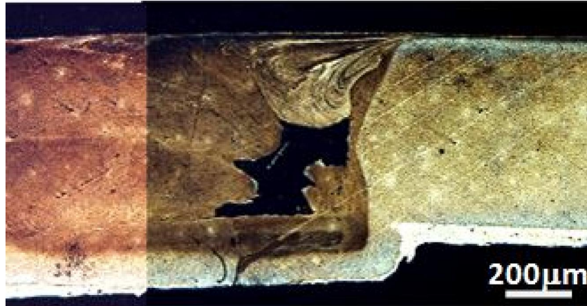
Figure 7. Macrograph of sample welded using 1800 rpm and 35.5mm/min
