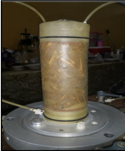
Figure 4. a. Preparation of Soil Sample S8 in Triaxial Cell.
