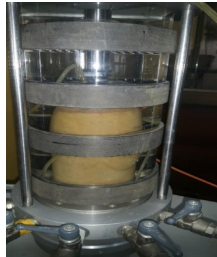
Figure 4. b. Shear failure in Soil Sample S1 in Triaxial Cell.
