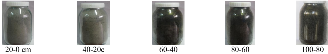
Figure 6- Rock appearance after in-situ combustion process
