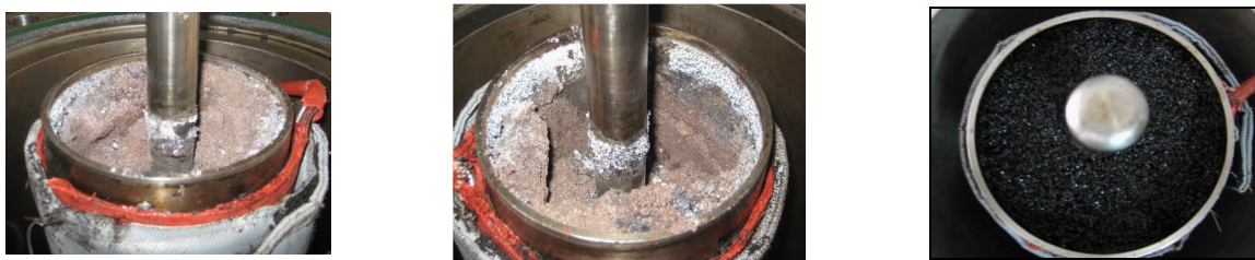
upper part of the combustion tube after combustion process upper part of the combustion tube after combustion process upper part of the combustion tube before combustion process
