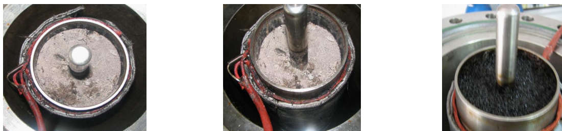
upper part of the combustion tube after combustion process upper part of the combustion tube after combustion process upper part of the combustion tube before combustion process
