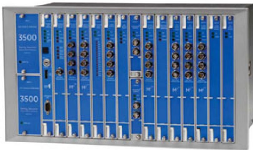
figure 6. bently Nevada 3500 series machinery monitoring system [1].
