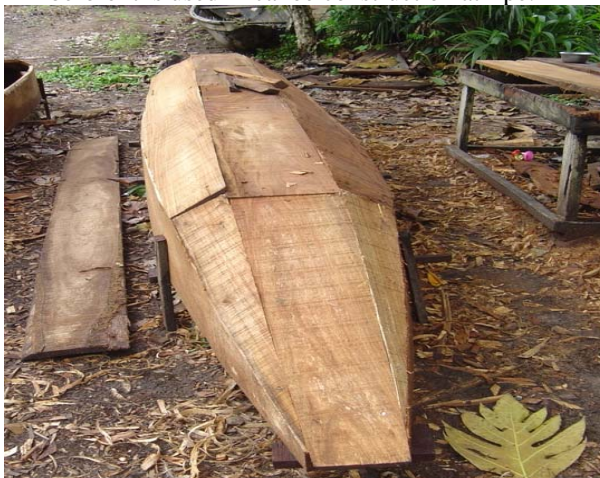
Plate 2.3: New constructed planked canoe at Epe (back hull)
