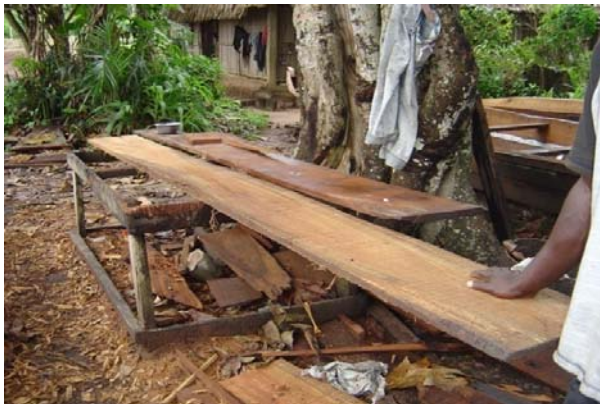
Plate 2.1: Planks placed on attender for framing before it is used in canoe construction at Epe.
